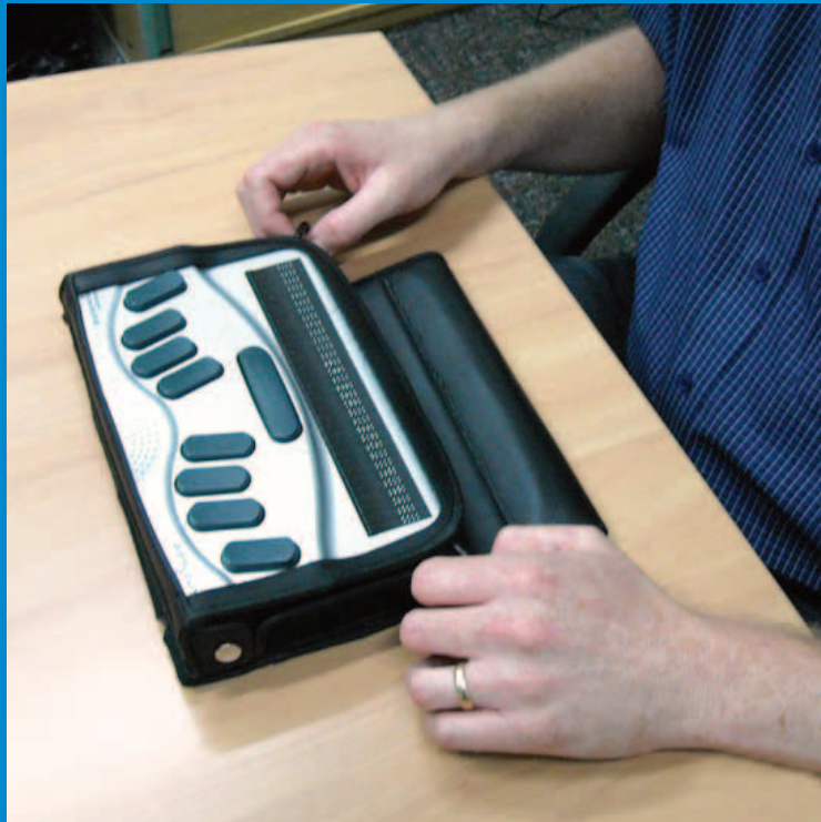
The Braille note reader has many of the functions of a conventional laptop. Through the nine key Braille keyboard, users can create Braille or Word documents or output to voice.
